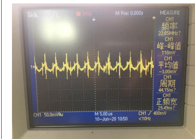
Noise ( V_{in}=48V , I_o=2A , 5~20MHz bandwidth)
