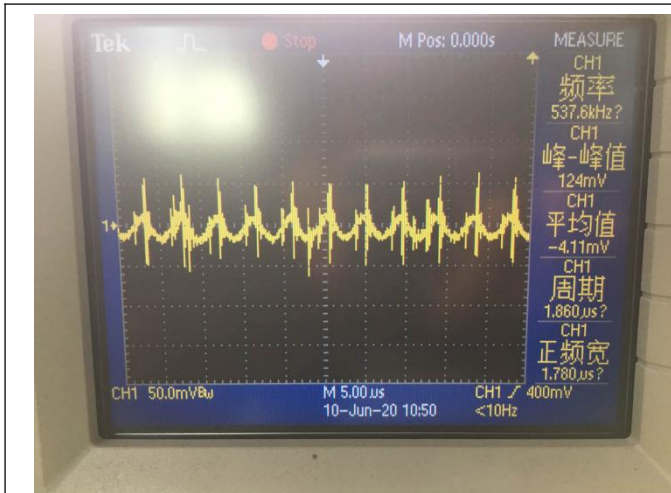
Noise ( V_{in}=42V , I_o=2A , 5~20MHz bandwidth)
