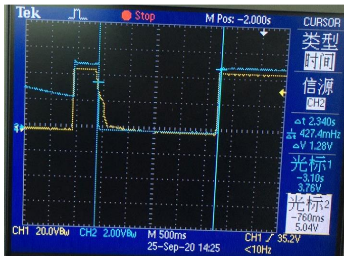
Output response & load (5V / 0.01A)
