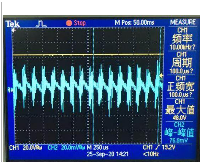
Noise (VIN = 48V, IO = 0.01A, 5 ~ 20MHz bandwidth)
