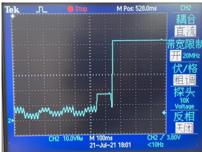
Noise (VIN = 48V, IO = 1A, 5 ~ 20MHz bandwidth)
