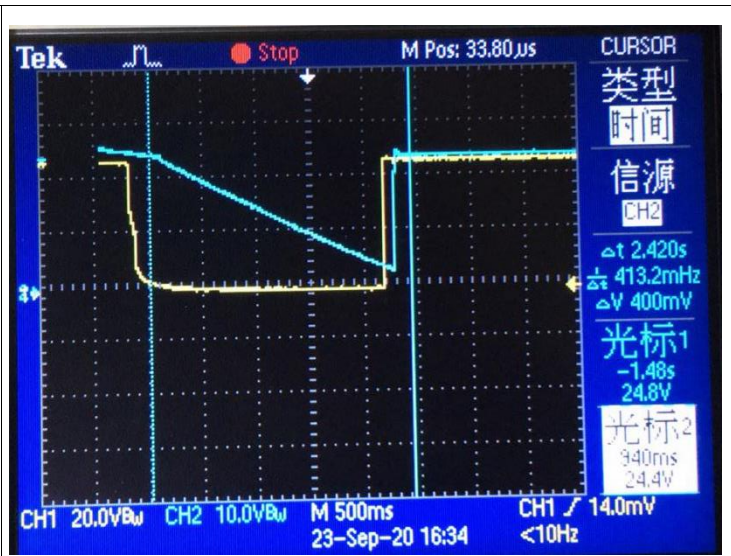
Output response & load (24V / 0.01A)
